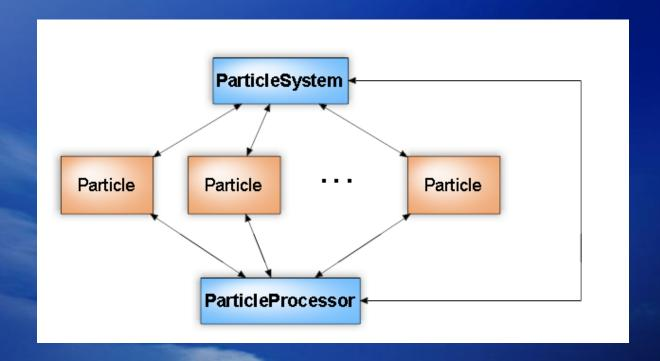
In our designment, the geometric information of a particle, like the vertex buffer or texture coordinate buffer which will be directly used to display those particles in the screen, is not stored in the Particle itself, but the ParticleSystem.
