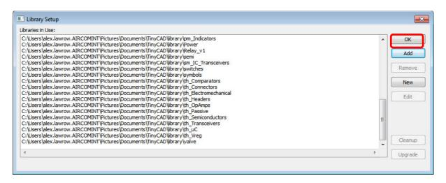
The symbol files provided with VeroRoute will probably be updated and expanded with new releases of the software. In order to use the latest symbols you must first remove any existing VeroRoute symbols from TinyCAD using the Library Setup dialog, and then add the new ones. The process is not automatic unfortunately.
