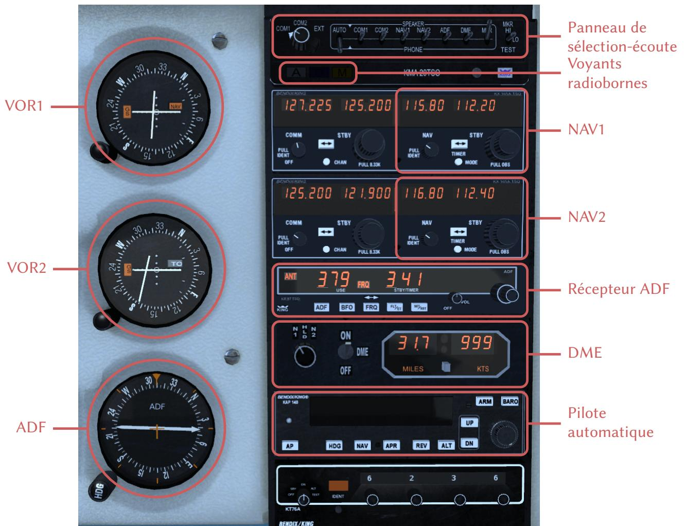
FIGURE 10.4 – IFR navigation instruments
